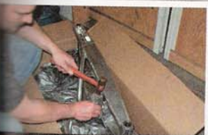
They are installing the pivot bearings into the Trac Dynamics swingarm. The high-quality arms have everything you need, and you can use the box it comes in to cushion the arm during installation of the bearings.
